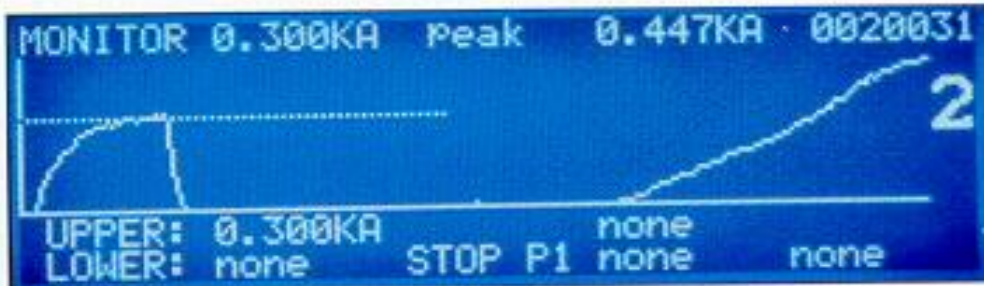
Monitor Screen – First pulse time automatically compensates for varying levels of oxides.
